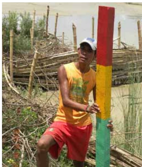
Photo 8: Three colored pole (Level 1, green: Alert/Standby/Ready-Level 2, yellow: Preparation "Get Set"-Level 3: Evacuation-Red).
