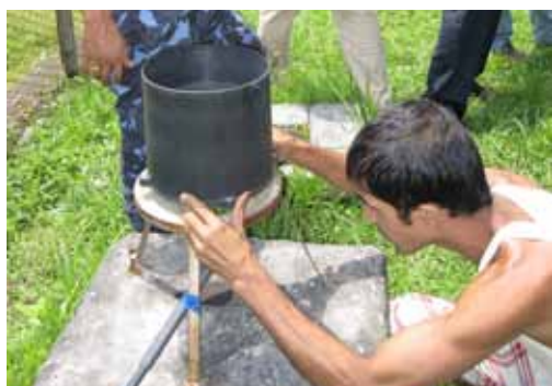
Photo 10: SEWIN_DHM_training-Automatic tipping bucket.
